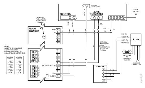
Figure 15. Connection of AAV Unit When Using a 4285 or 4286 Phone Module
